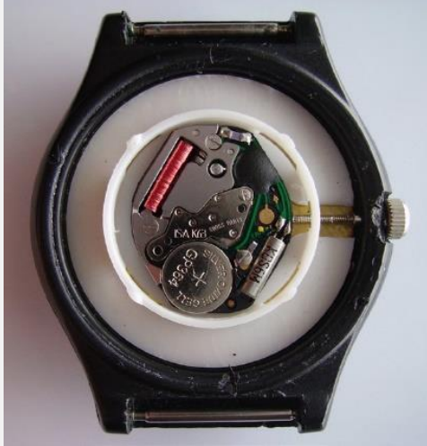
A battery powered quartz watch movement.
